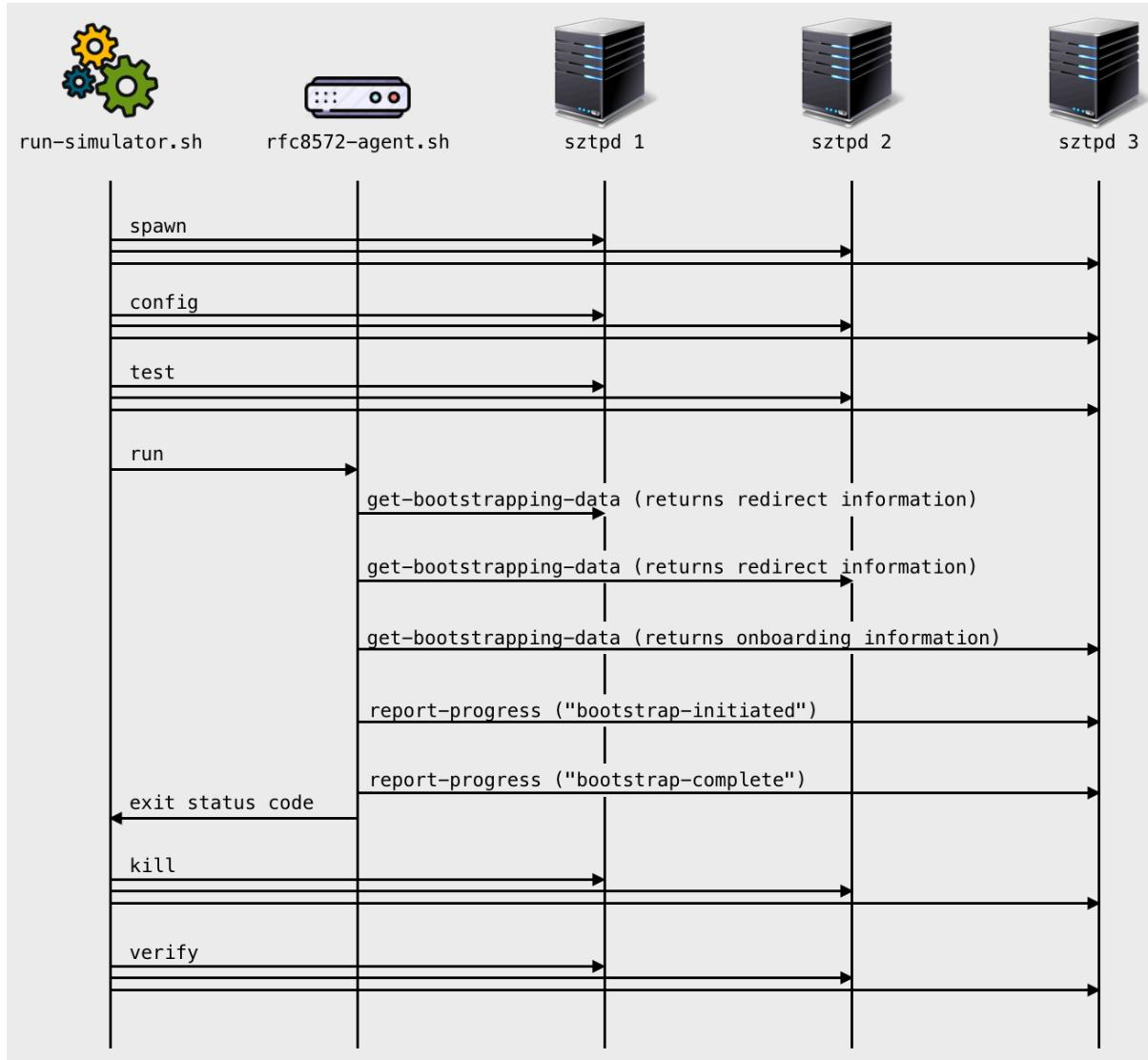
The simulator (i.e., the script `run-sztpd-test.sh`) performs the following steps:
